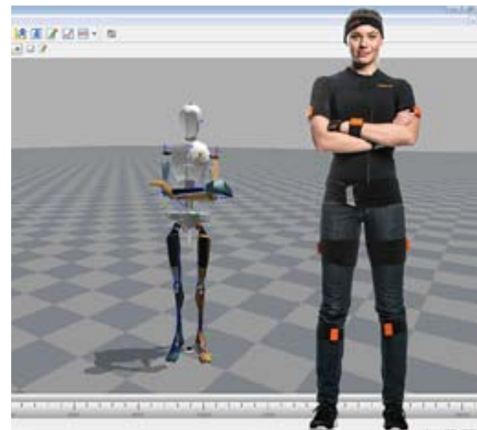
Figure 1: Xsens MVN Awinda (inertial motion capture) suit.
